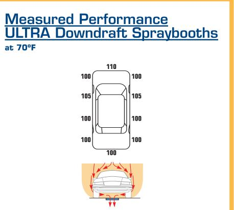
All measurements should be made with a non-averaging velometer. Measure at door handle height, completely around vehicle.
