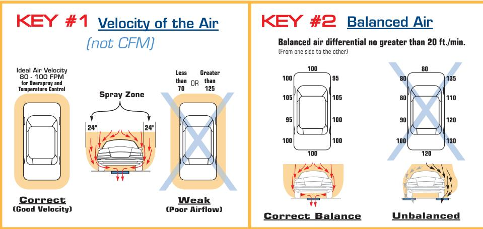
All measurements should be made with a non-averaging velometer. Measure at door handle height, completely around vehicle.
